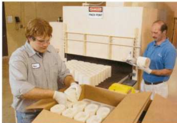
Each catalyst undergoes a series of automatic quality checks, along with a final visual inspection prior to packaging and shipping.
