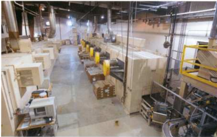
The new catalyst manufacturing system combines 20 different steps, including five weight checks, applications of the precious metal washcoat, flow checking, automated laser 2-D matrix bar code labeling and furnace drying into one continuous flow.
